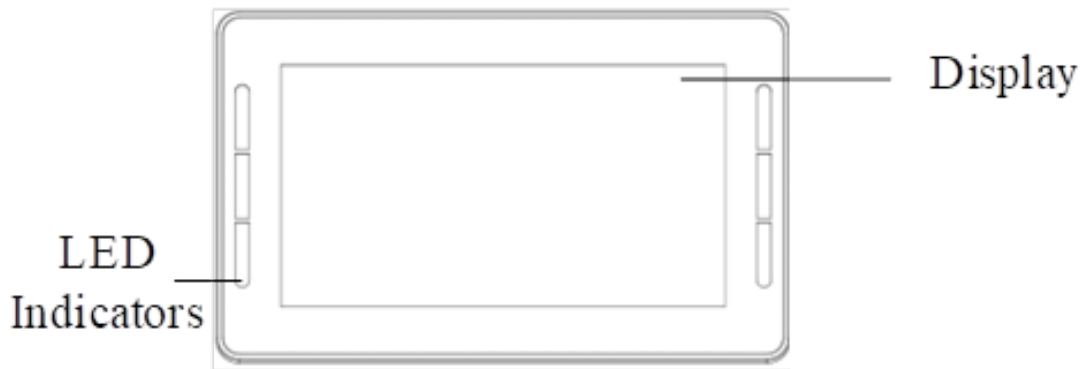
Figure7- 1: UPS operator control and display panel
